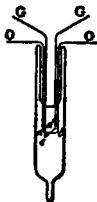
FIG. 48.—Tellurium-Bismuth Vacuum Thermoelectric Oscillator. a , b , constantan wire; c , d , platinum wire; e , f , thermo-junction; g , h , damping of the train of oscillations, that galvanometer terminals; i , j , antenna and earth terminals.
