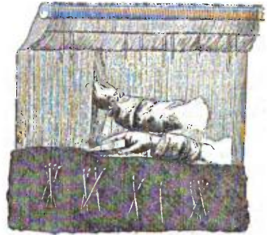
FIG. 2.—Gobelines tapestry-weaving, showing (a) the left hand of the weaver pulling forward (c) a group of warp threads, into which with (b) the comb in his right hand he is compressing at point (d) the weft threads which have been passed around and in between the warp threads; (e) are various bobbins, hanging at rest, suspended by their weft threads; and (f) is the tapestry as woven and compressed.
